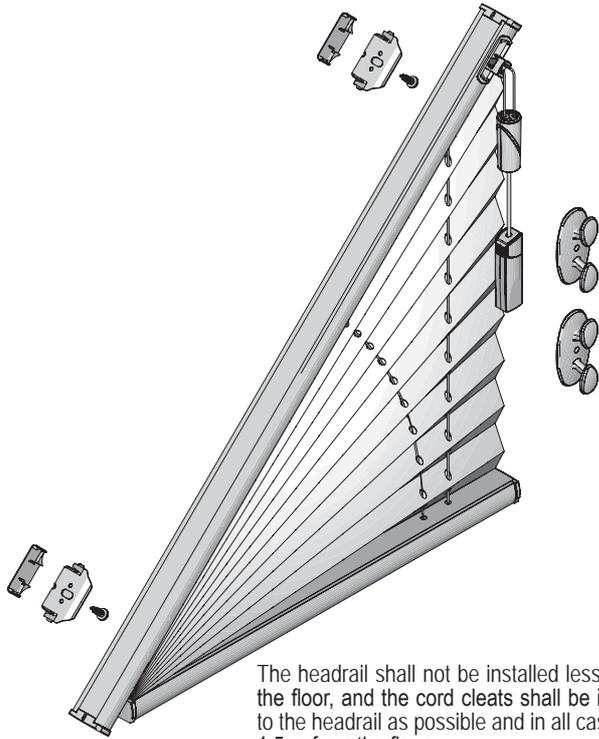
The headrail shall not be installed less than 1,5 m from the floor, and the cord cleats shall be installed as close to the headrail as possible and in all cases, not less than 1,5 m from the floor.
